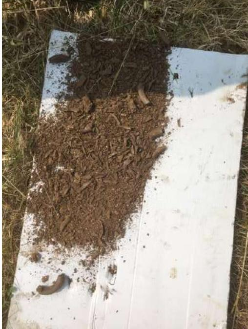
A photograph of a white rectangular tray containing a dark brown, granular soil sample. The sample is heavily mixed with organic debris, including small twigs and leaves, and appears to be a limon argileux facies. |
