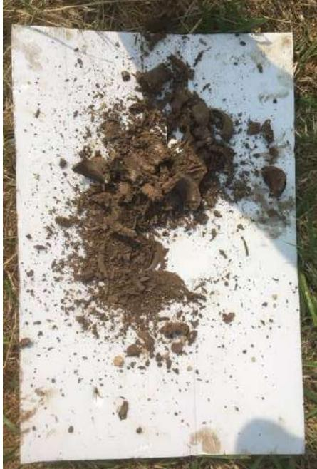
A photograph of a white rectangular tray containing a dark brown, granular soil sample. The sample is heavily mixed with organic debris, including small twigs and leaves, and appears to be a limon argileux facies.  |
