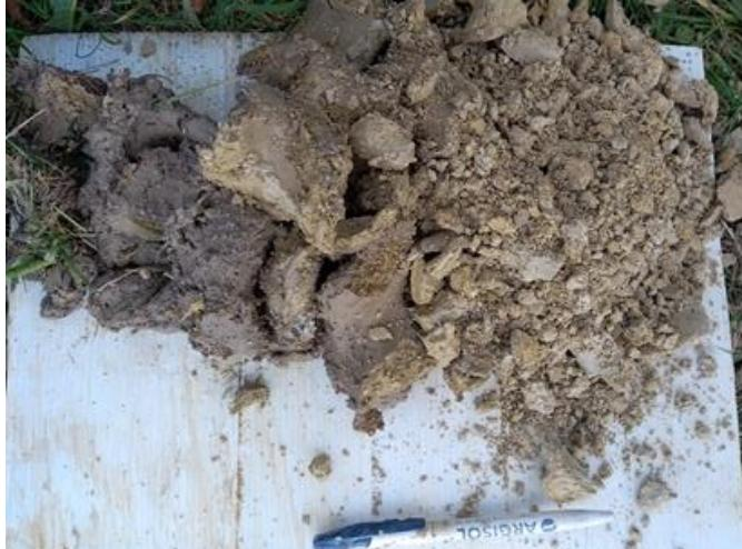
A photograph showing a dark brown, crumbly soil sample from test T6. The sample is resting on a white plastic tray with the brand name 'ARGISOL' printed on it. The soil texture appears similar to sample T5, with a mix of fine particles and larger rock fragments. |
