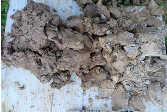
A photograph showing a dark brown, crumbly soil sample from test T5. The sample is resting on a white plastic tray with the brand name 'ARGISOL' printed on it. The soil has a mix of fine particles and larger, angular rock fragments.                                |
